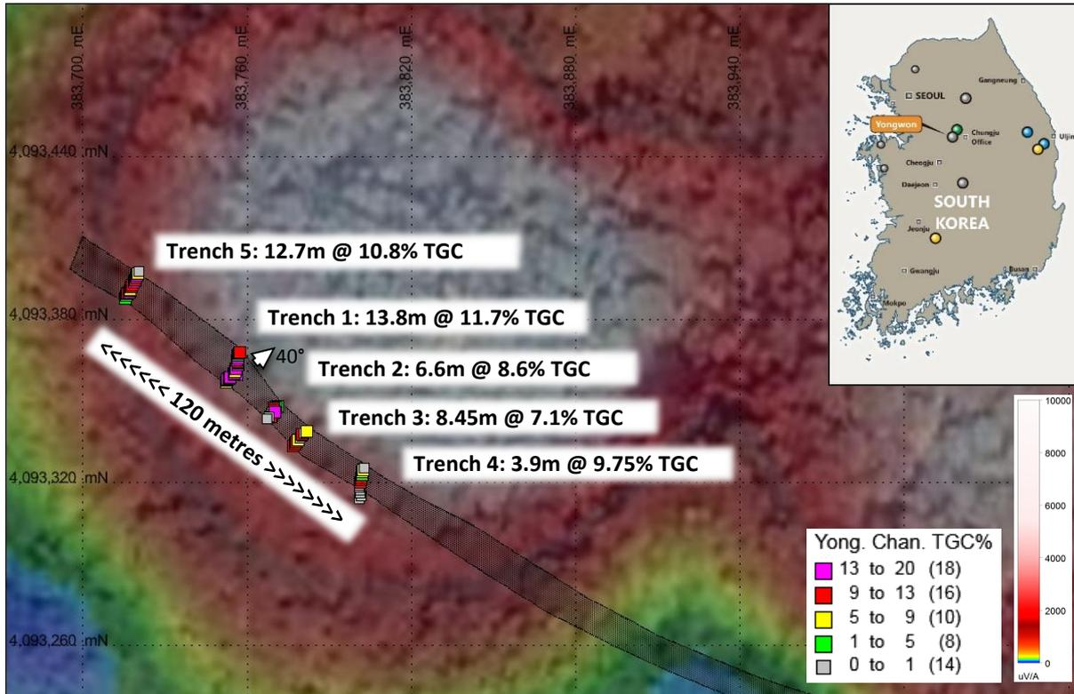
Figure 1: Mapped/interpreted Yongwon Graphite Unit (grey) and channel sampling results on EM imagery<sup>D4</sup>
